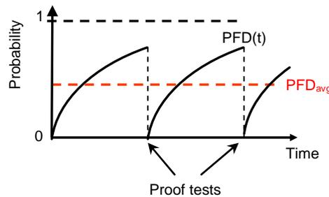
One can see that the SIL value of a SIF determined by the failure rates of the components of a SIF and by the proof testing. If the SIF exists and failure rates are given and proof testing is the only method to increase the safety integrity
