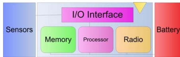
Figure 2. Sensor Node Architecture
