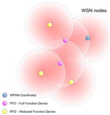
Figure 3. Typical wireless sensor network (WSN)
