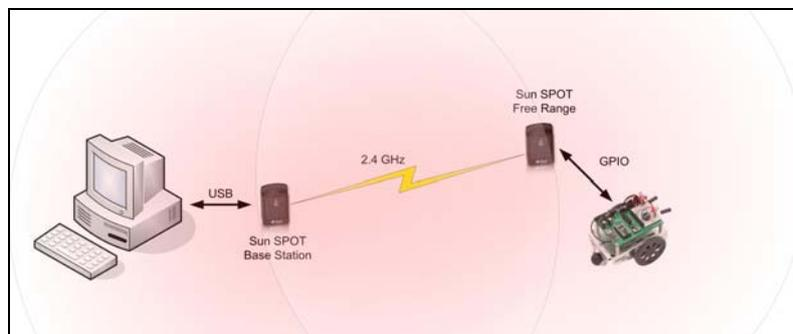
Figure 7. Connection of the system
