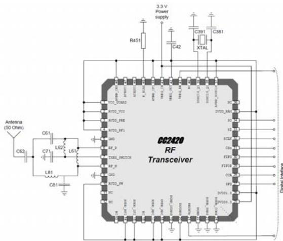
Figure 4. Typical application circuit for CC2420
