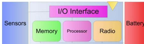
Figure 2. Sensor Node Architecture
