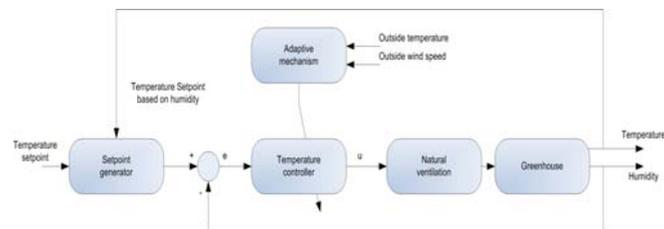
Figure 4. Temperature controller
