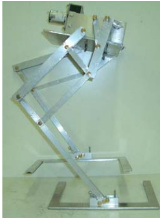
Figure 8 Prototype of a biped walking robot at LARM
