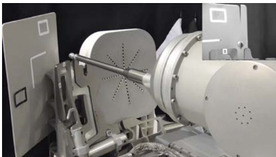
ROKVISS robot with experimental task board
