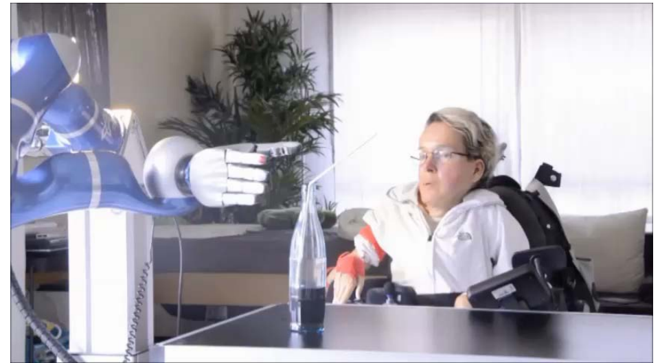
EMG-Interface for arm-position & hand-actions
