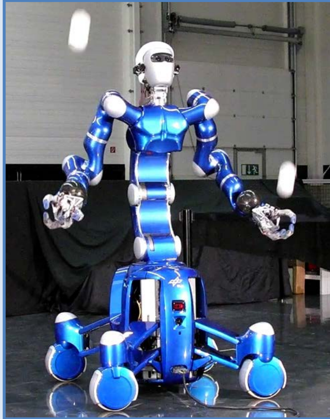
JUSTIN and TORO are based on LWR III – Torque Controlled Flexible Joint Technology
