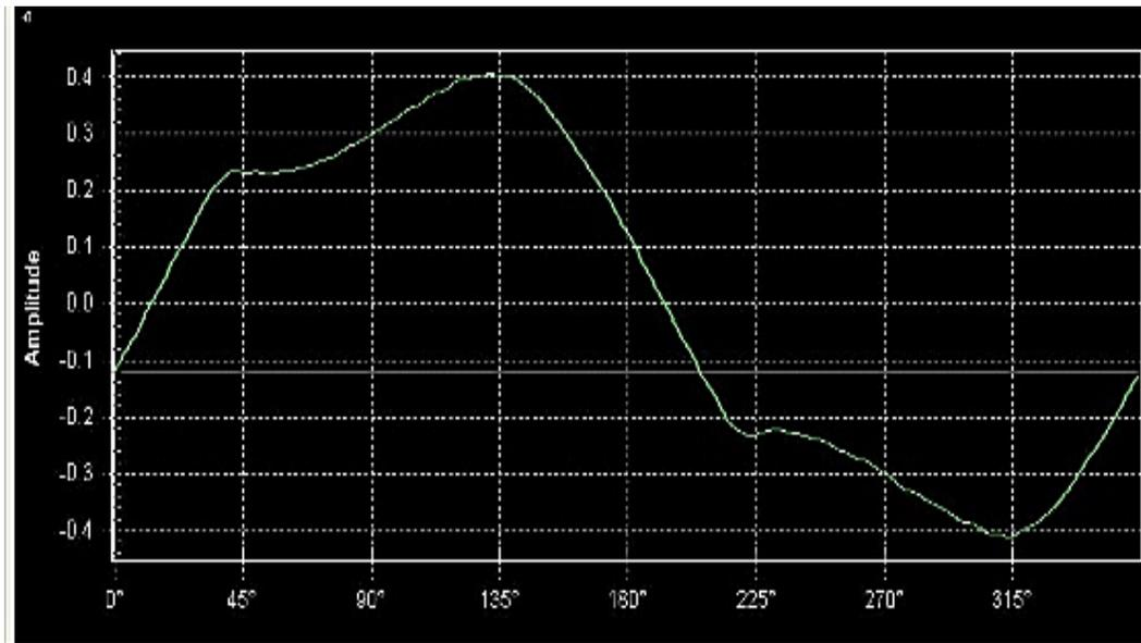
Fig. 2 The waveform of the current drawn for a sinusoidal supply voltage.
