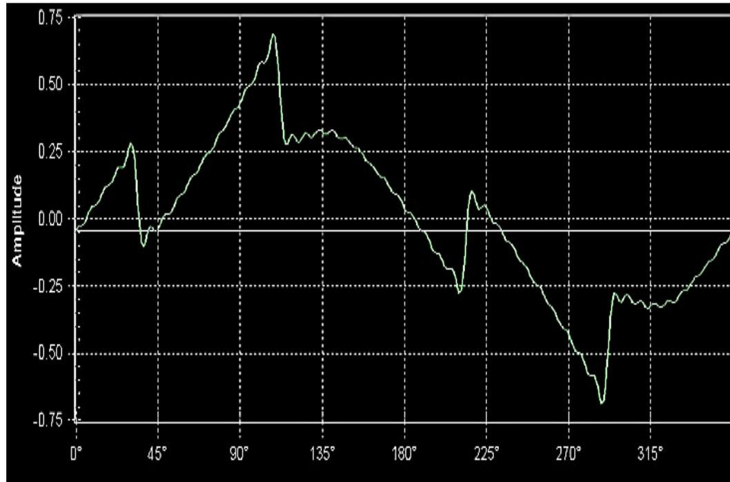
Fig. 4 The waveform of the current drawn for a 10% clipped supply voltage.
