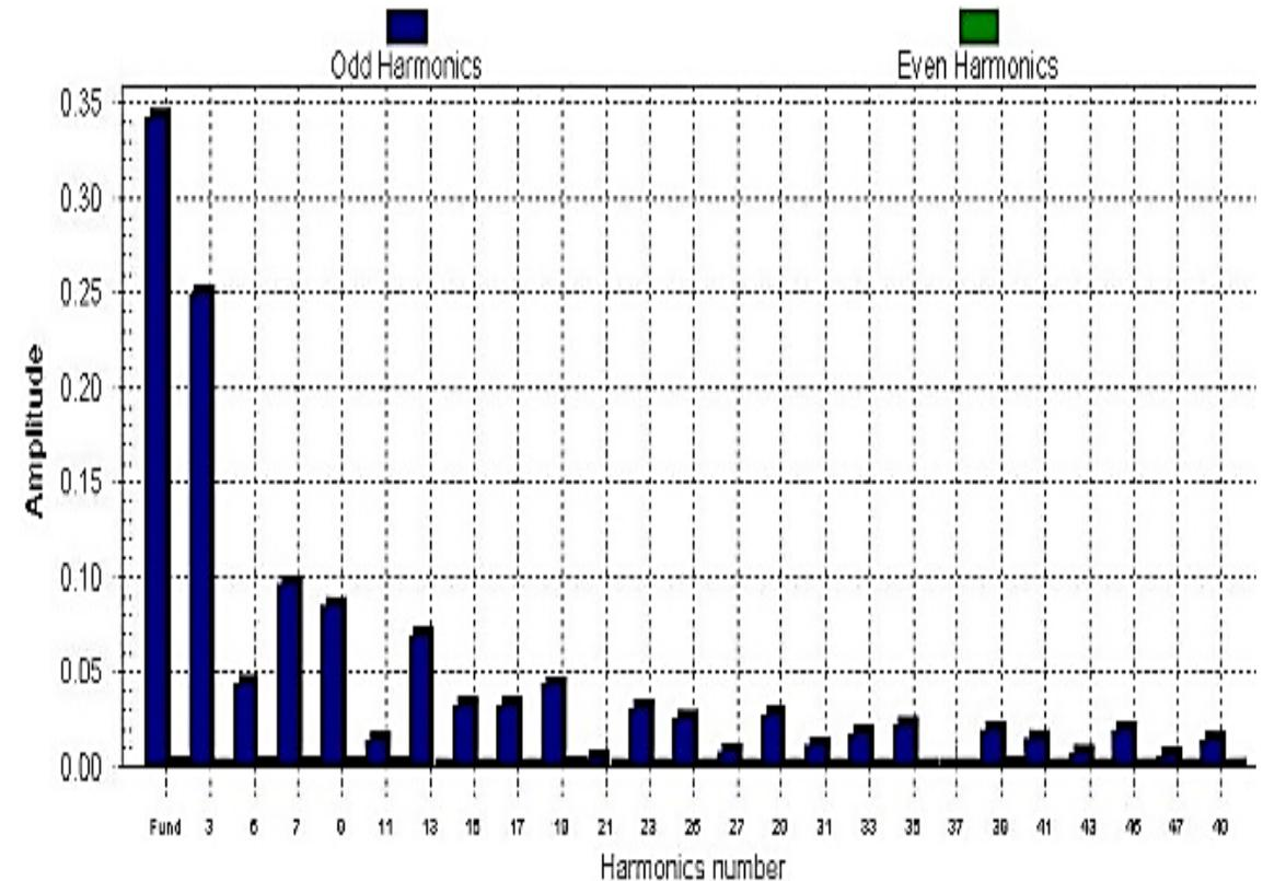
Fig. 12 Harmonic spectrum of the current drawn for a 20% clipped supply voltage.
