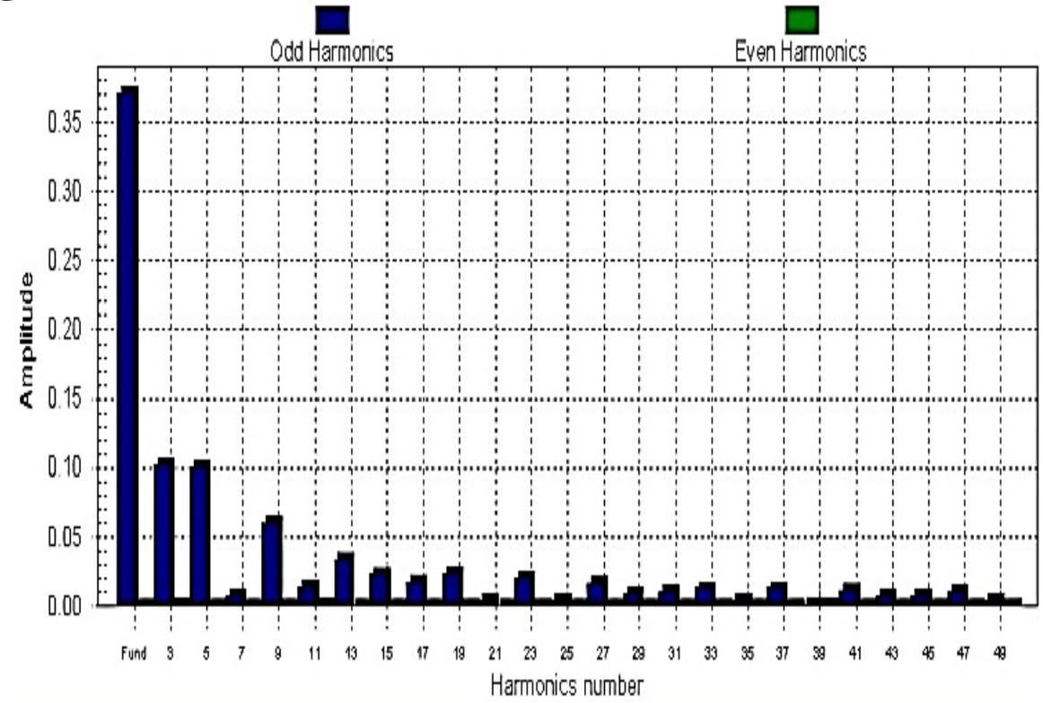
Fig. 7 Harmonic spectrum of the current drawn for a 10% clipped supply voltage.
