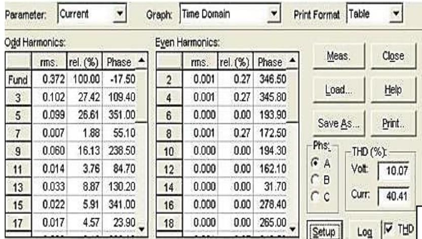
Fig. 5 Upper part of the harmonic analysis window of the current drawn for a 10% clipped supply voltage.
