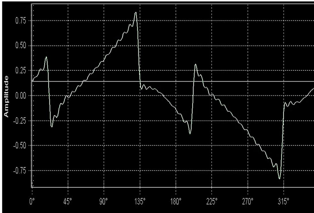
Fig. 9 The waveform of the current drawn for a 20% clipped supply voltage.
