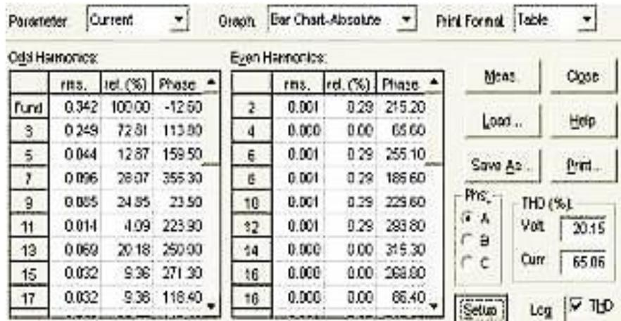
Fig. 10 Upper part of the harmonic analysis window of the current drawn for a 20% clipped supply voltage.
