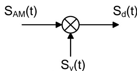
$$S_d(t) = S_{AM}(t) \cdot \cos(\omega_v t + \varphi) = a(t) \cos(\omega_v t) \cdot \cos(\omega_v t + \varphi) = \frac{a(t)}{2} \cdot \cos \varphi + \frac{a(t)}{2} \cdot \cos(2\omega_v t + \varphi)$$
