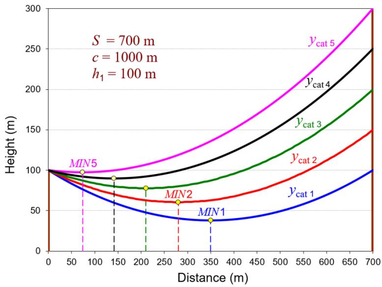
Catenary curves in the spans of the same length but with different inclinations, shown in the same figure related to a numerical example
