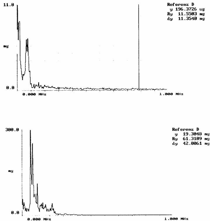
Fig.1. AE spectrum of sharp and worn 1.5mm diameter twist drill (material KO36 feed 25mm/min, 2500 rev/min)
