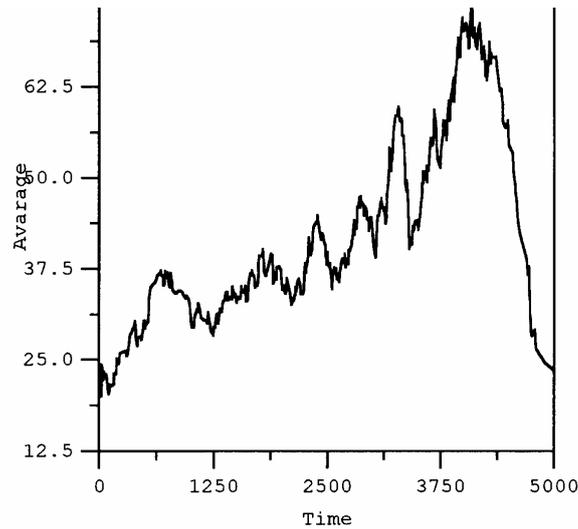
Fig.4. The processed AE signal in case of tool failure
