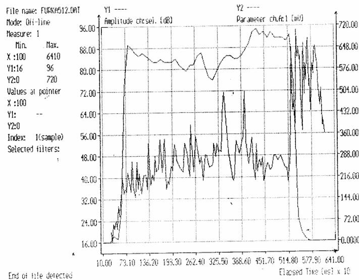
Fig. 3. AE activity and feedforce during tool failure
