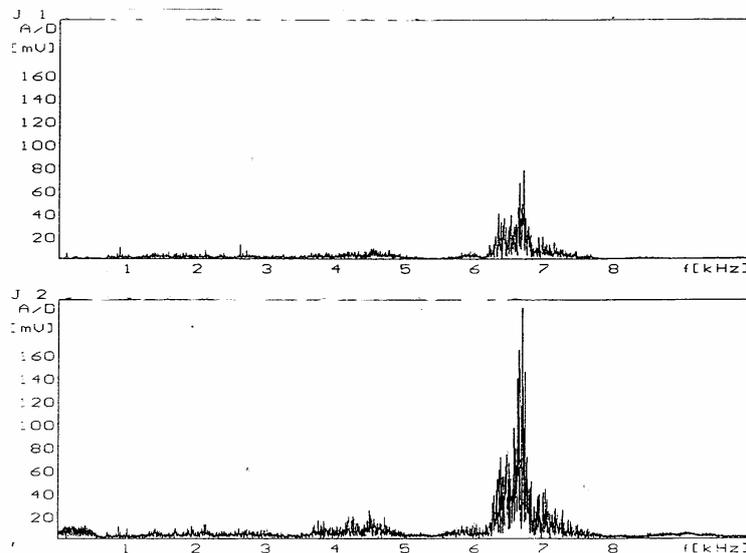
Fig.2. Vibration spectrum of a 1.5 mm twist drill
