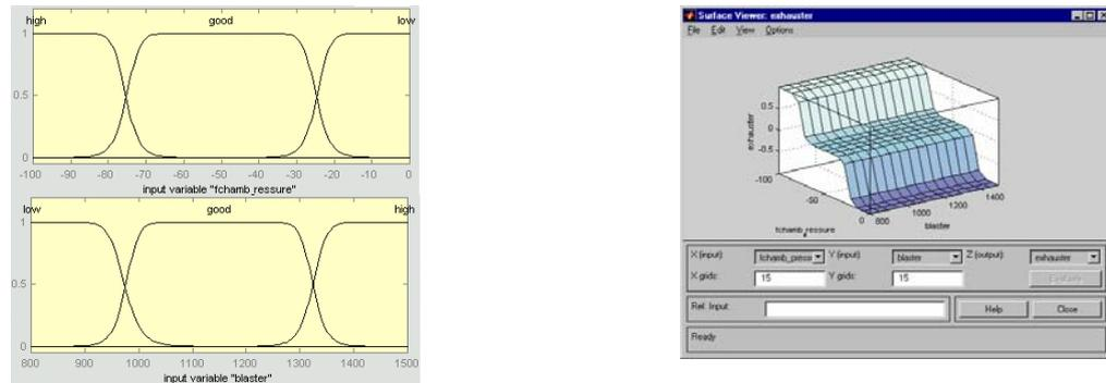
**Figure 2.9. MFs of FIS for control of revolution number of exhauster ventilator**
