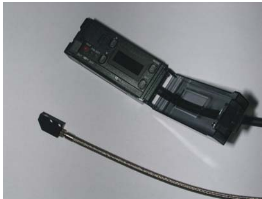
Figure 2 Colour Sensor CZ-11 and evaluation unit CZ-K1(P)
