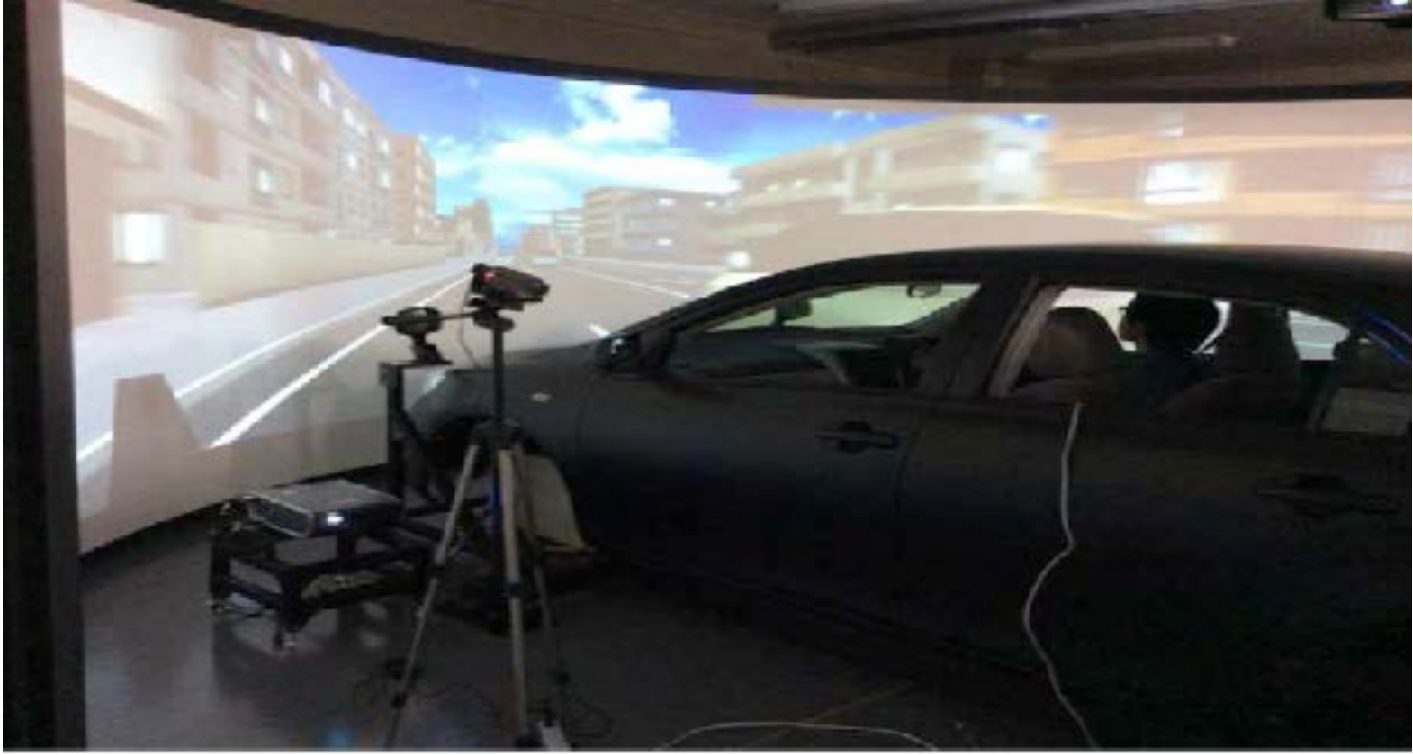
Fig. 2: Drive simulation measuring subjective driver profiles
