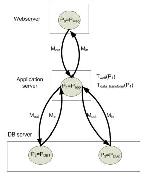
Figure 2 Process interaction graph of a three-tier architecture
