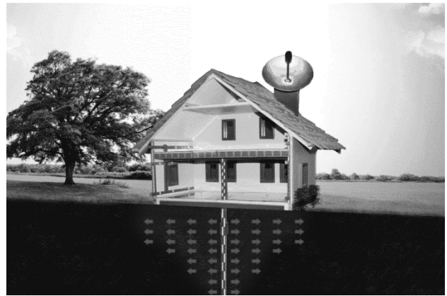
Figure 6. A technical solution to transport solar energy from solar collectors to the vertical DHE
