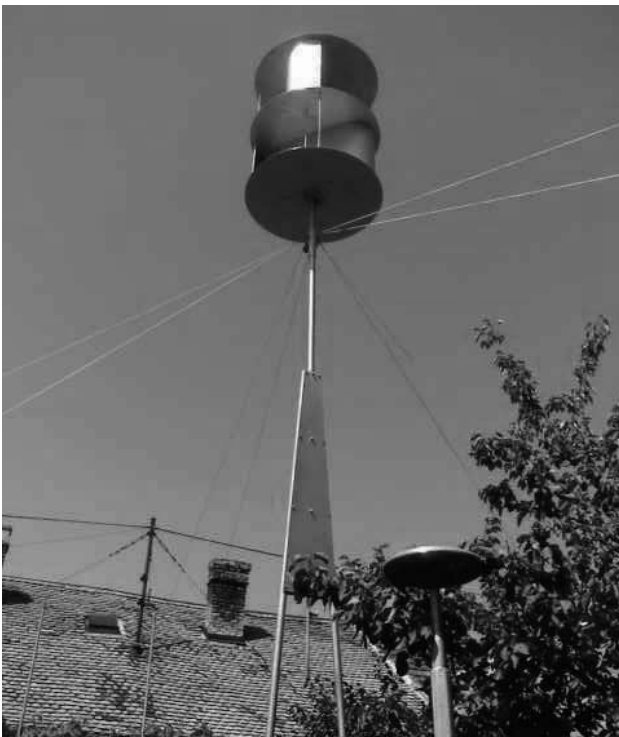
Figure 2. The wind turbine built by the authors.
