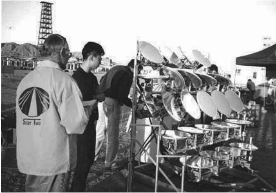
Figure 1. Stretched membrane concentrator cluster and focally positioned high temperature receiver.
