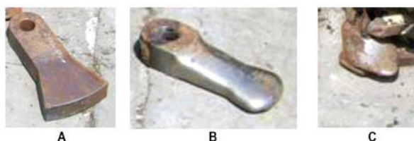
Figure 7. Abrasion of the hammers
