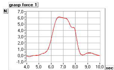
Figure 5 Plots of the force measured by sensor 1 during a cylindrical grasping of an object made of compliant plastic with LARM Hand of Fig. 2
