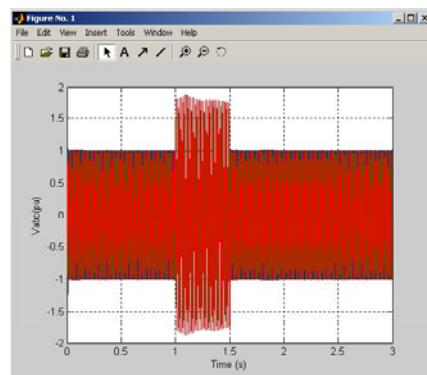
Figure 4. Vabc 3-phase voltage (pu).
