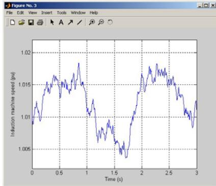
Figure 12. Asynchronous machine's speed (pu).
