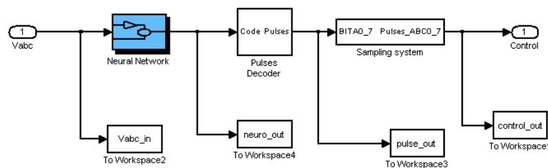
Figure 3. The frequency regulator based on a neural network.
