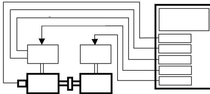
The neuro-fuzzy controller is implemented on a DSP (TMS320C31@50MHz) equipped with position encoder, 16 bit analogue-digital converters (ADC) and digital-analogue converters (DAC). The armature current is measured with the aid of a current transducer. The armature voltage is also measured with the aid of a current transducer using a resistor in parallel with the servomotor. The shaft encoder type is ROD426 and its precision is very low,  $N_0=2500$
