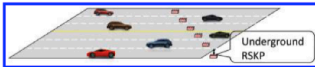
Fig. 6. Key donation with RSKP equipment embedded in the pavement. RSKPs are located underground of each lane.
