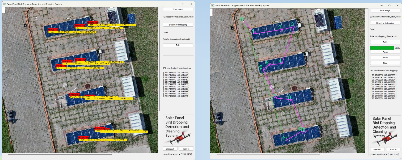
Fig. 12. User interface for bird dropping GPS coordinate detection and generation of optimal cleaning route..
