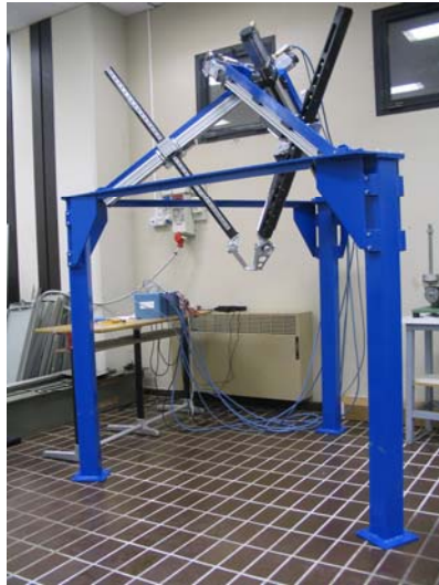
Figure 10 Prototype of the 3-CPU translating parallel machine
