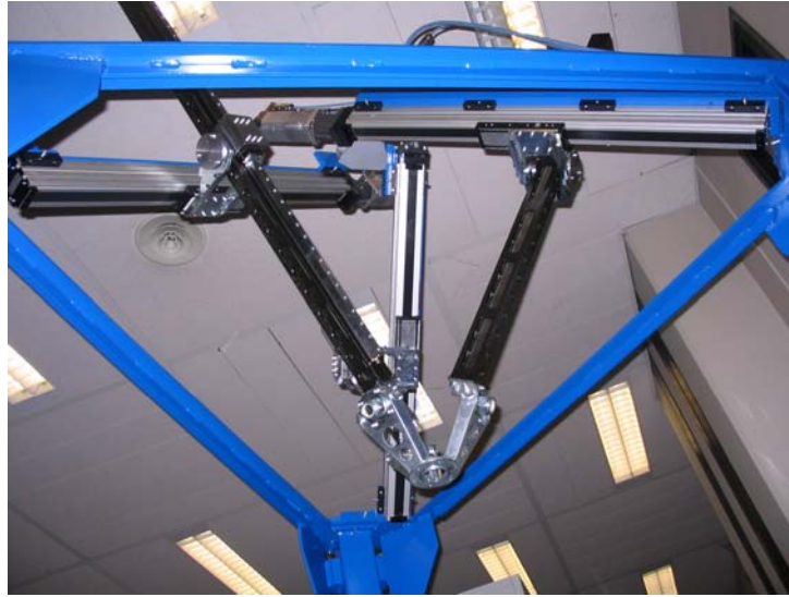
Figure 6 CPU kinematic structure of the limbs
