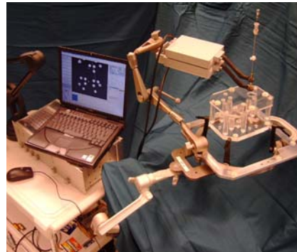
Figure 4 Test setup for NS interventions; phantom attached to CRW frame
