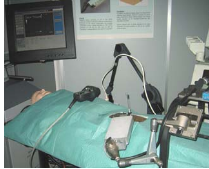
Figure 3 Test setup for US-guided biopsies
